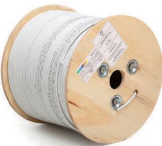
STP cable 4x2xAWG23, Category 6<sub>A</sub>, 550 MHz, LSOH, Euroclass D<sub>ca</sub> - s2, d2, a1
