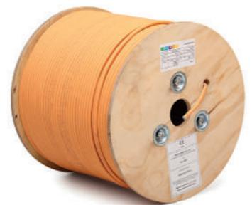
STP cable 4x2xAWG23, Category 6<sub>A</sub>, 550 MHz, LSOH, Euroclass B2<sub>ca</sub> - s1a, d1, a1
