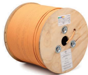
STP cable 4x2xAWG23, Category 6<sub>A</sub>, 550 MHz, LSOH, Euroclass B2<sub>ca</sub> - s1a, d1, a1
