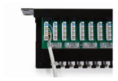
Fasten cable ties for additional strain relief.
