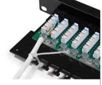
Fasten the screws through metal case to hold tightly down for two cable jackets in the same time.
