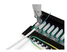
Punch down wires with LSA-tool.
