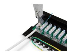
Punch down wires with LSA-tool.
