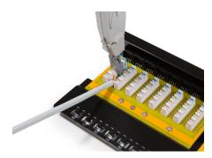
Punch down wires with impact tool.
