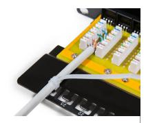
Follow the IDC colour-code for T568A or T568B wiring and set pairs into proper position.
