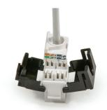
Put the cap on the IDC tower. The arrows on Close the jaw until it clicks into place. the jack and the cap should face the same direction. Put the cap into the position.
