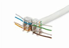
Lay the wires to their correct positions based on the color code (T568A/T568B).
