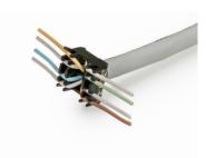
Lay the wires to their correct positions based on the color code (T568A/T568B).
