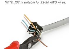
Cut the excess wires off. The tips of the wires should protrude no more than 0,5 mm.
